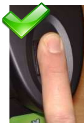
Finger placed correctly on the sensor glass. Slight pressure is necessary.
