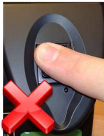
Finger placed skew on the sensor glass.
