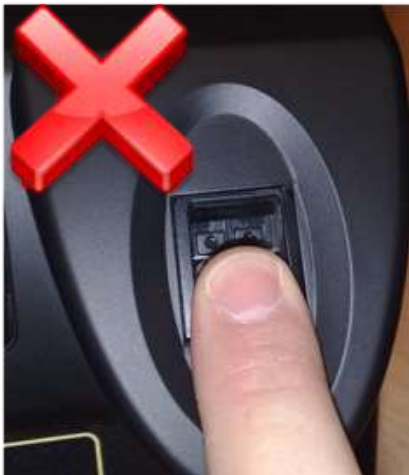
Finger placed too low on the sensor glass.
