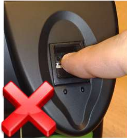
Only finger tip placed on the sensor glass.
