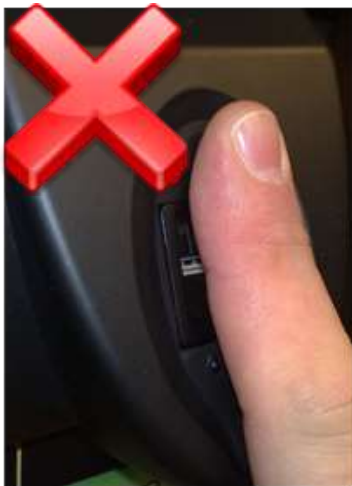
Finger placed too high on the sensor glass.
