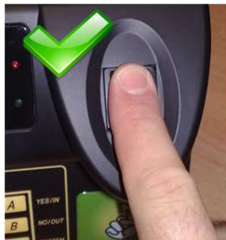
Finger placed correctly on the sensor glass. Slight pressure is necessary.
