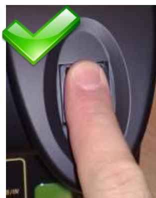
Finger placed correctly on the sensor glass. Slight pressure is necessary.
